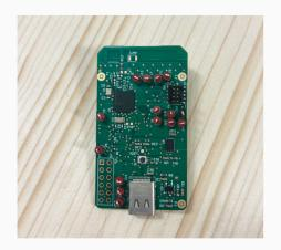
Prototype PCB used on a medical device company to collect users' activity information. This project was developed to collect the patient activity through an IMU sensor, store it on a flash memory and then transfer everything to a software via Bluetooth. On this PCB we have a lot of test points (red pins) to test all the communications between the different devices.
